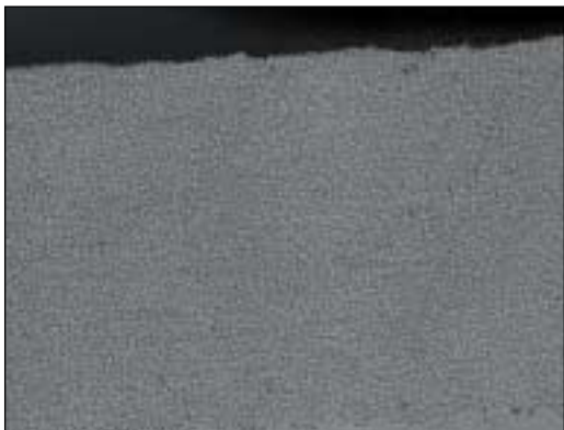
HVOF tungsten carbide has a bonding strength to the substrate of 80 MPa (10 ksi).
